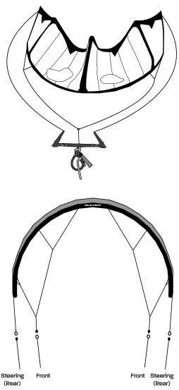
WARNING: Naish flying lines and bridles feature foolproof connectors to reduce the risk of incorrect connection between front and steering (rear) line connection points. Be sure to always use authentic Naish flying lines and bridles when using Naish kites and control systems.
