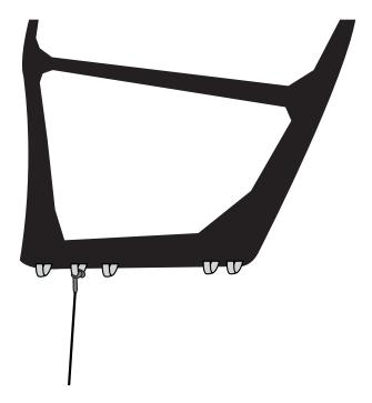
**A)** For increased bar pressure, move the back line connector to the forward attachment point.
