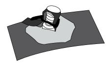
**B)** Open the strut valves to release the air from the struts.
