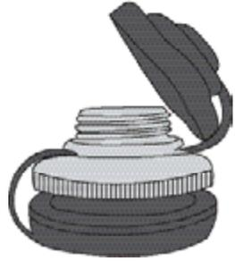
**G)** Insert the pump nozzle into the high flow valve opening.
